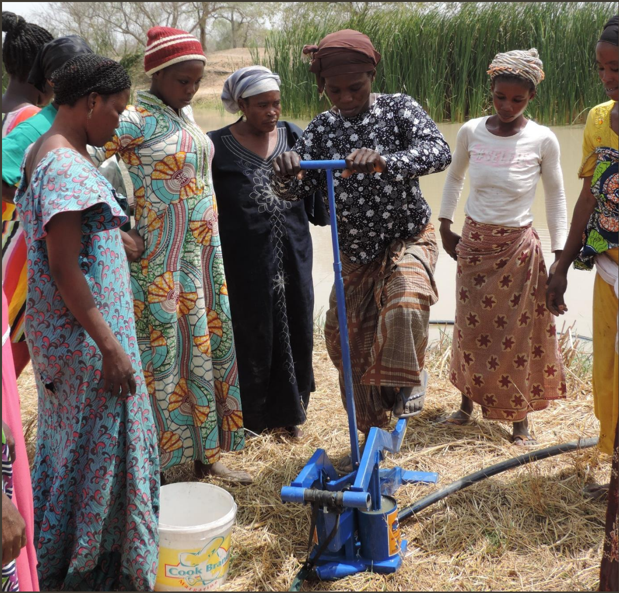
Photo: women testing the Money Maker pedal pump to reduce the time burden in watering their leafy green vegetable gardens that they cultivate jointly during the dry season.
