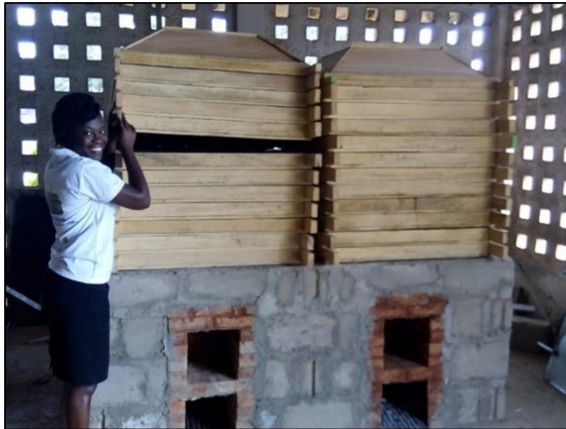
Figure 26 A double-unit Ahotor stove, offering lower-PAH levels and an improved energy efficiency
