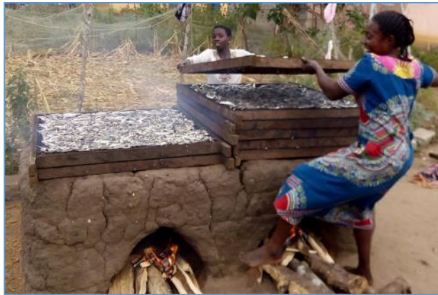
Figure 23 A Chorkor Stove in use. The same basic design is now used throughout West Africa
