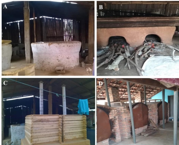
Figure 10 Types of ovens; (A) Circular ovens (B) Rectangular ovens (chorkor smoker) (C) Morrison stoves (D) Kosmos improved ovens
