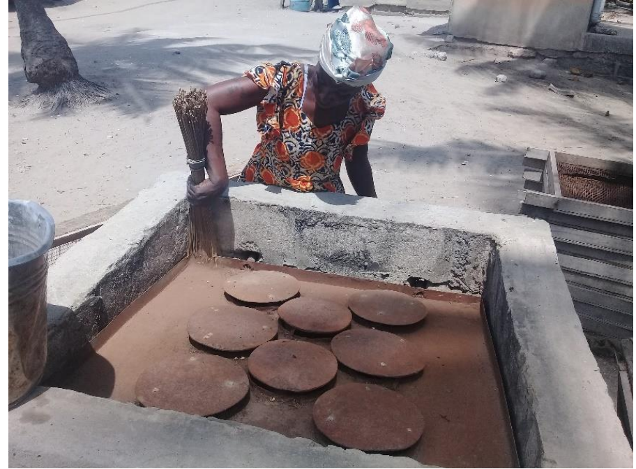
Figure 5: Madam Comfort Oklikah, cleaning the Fat collector on Ahotor Oven before using for smoking fish
