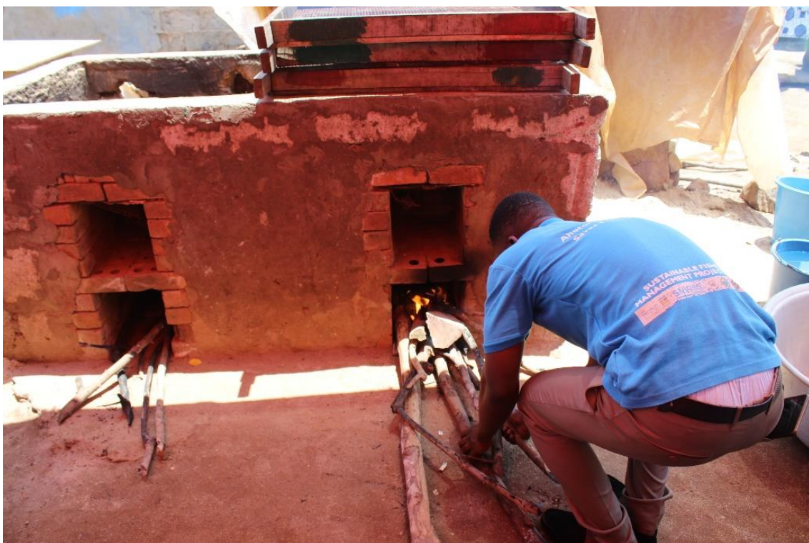
Figure 20: Ibrahim Nassam Community Liaison person of Apam, teaching processors how set fire on the Ahotor Oven
