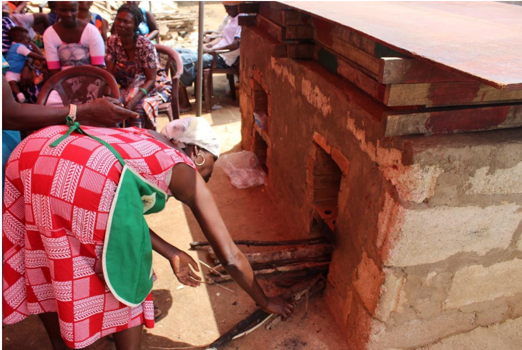
Figure 19: Madam Ellen Tetteh a fish processor from Apam arranging fire wood into grate in the combustion chamber of the Ahotor Oven.
