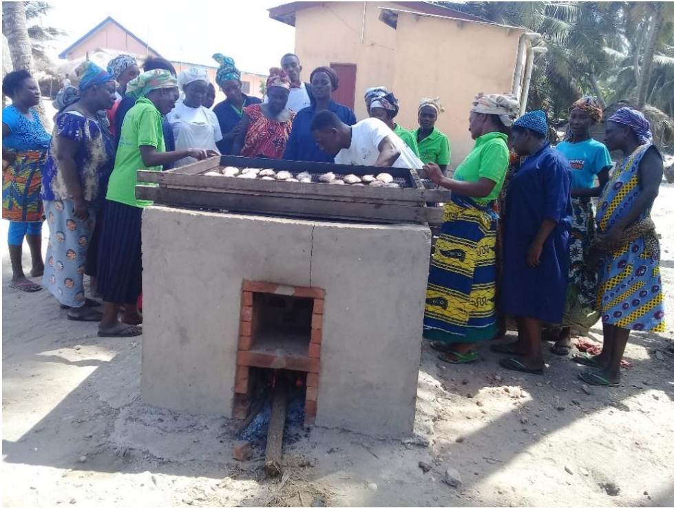
Figure 1: Fish processors at Warabeba learning how to use Ahotor Oven for smoking fish
