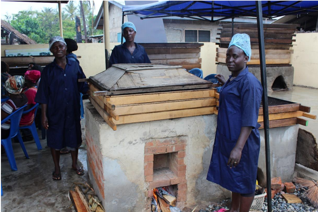
Figure 15: Ahotor Oven is being used to smoked fish at Tsokomey by some Processors.
