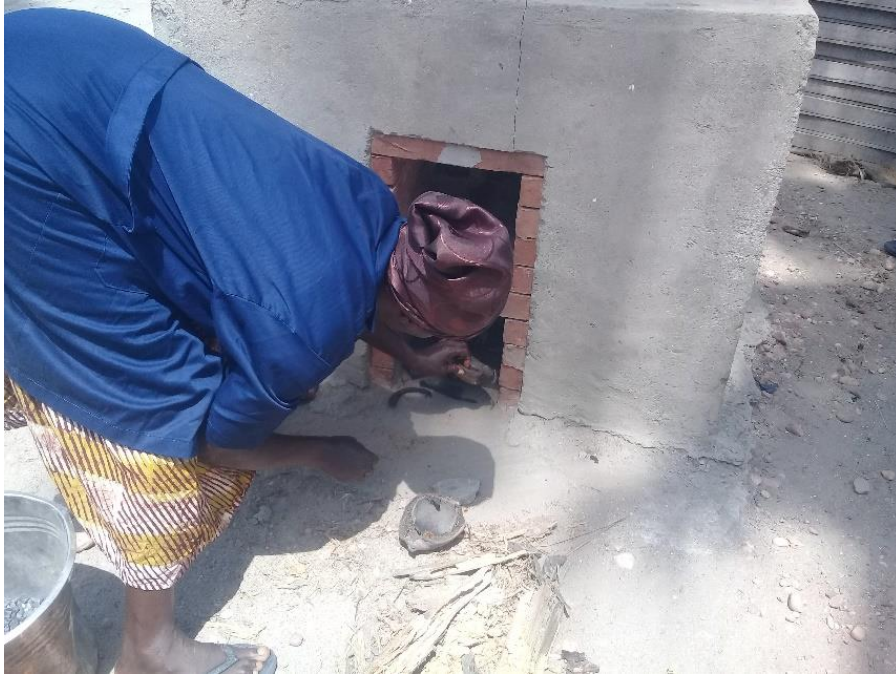
Figure 6: Madam Charity Gakor, setting fire in the Ahotor Oven for smoking fish
