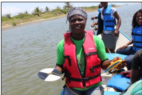
Figure 23: Left: Mr Godwin Hortor, using a bottom sampler to check for bottom water salinity; Right: Madam Bernice Bebli using secchi disk to check for water turbidity
