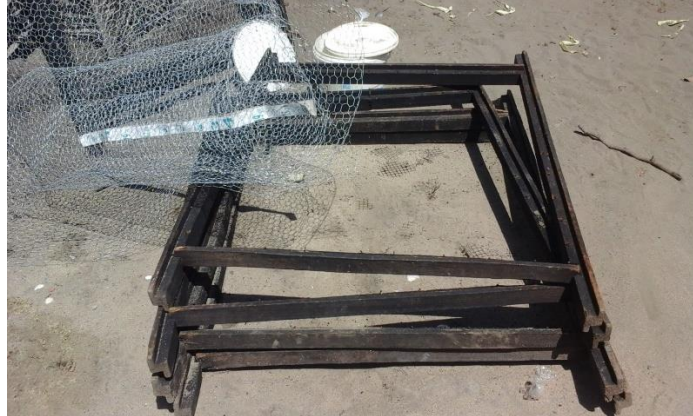
Figure 9: Damaged Morrison tray mesh, replaced with Chorkor tray mesh
