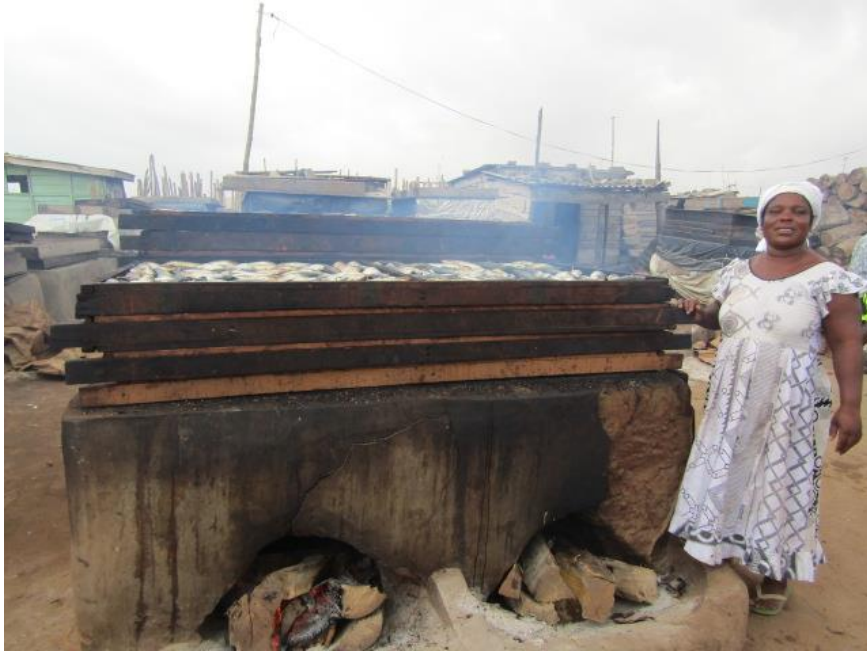
Figure 7. Chorkor oven with its combustion chamber fully filled with fuelwood at Chorkor
