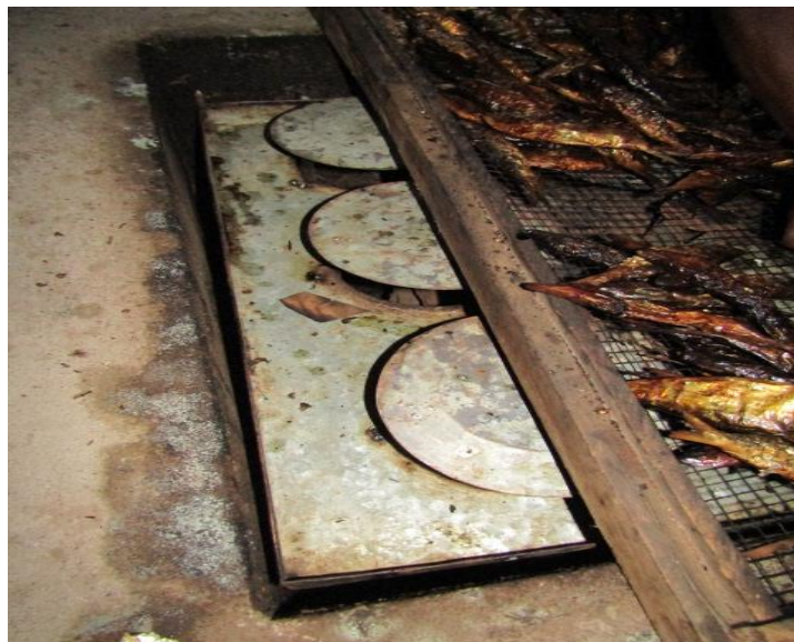
Figure 8. Ahotor oven showing distance between fish tray and fat collector
