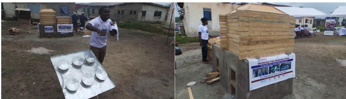
Figure 34. Mr. Emmanuel Kwarteng, from SNV demonstrating how the fat collector in the improved AHOTOR works
