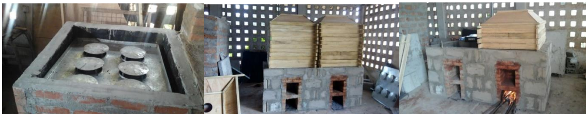
Figure 32. Pictures showing a newly built AHOTOR Oven
