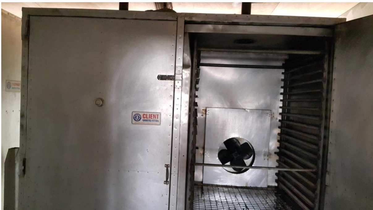
Plate 5 Abuesi Gas Fish Smoker – Top showing both chambers closed and Below showing one chamber opened.
