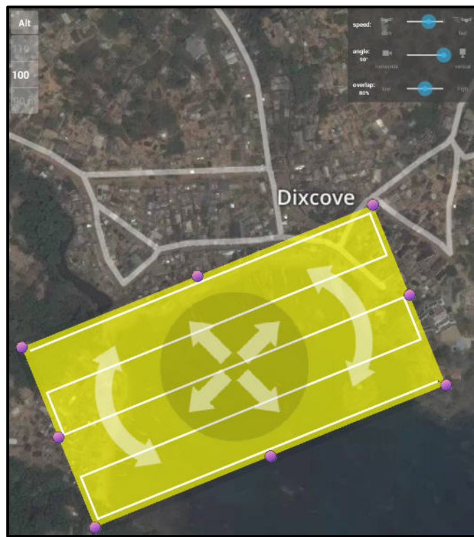
Figure 3 User interface for the Pix4D Capture App, a UAV Mission Planning and Control (MP&C) utility.
