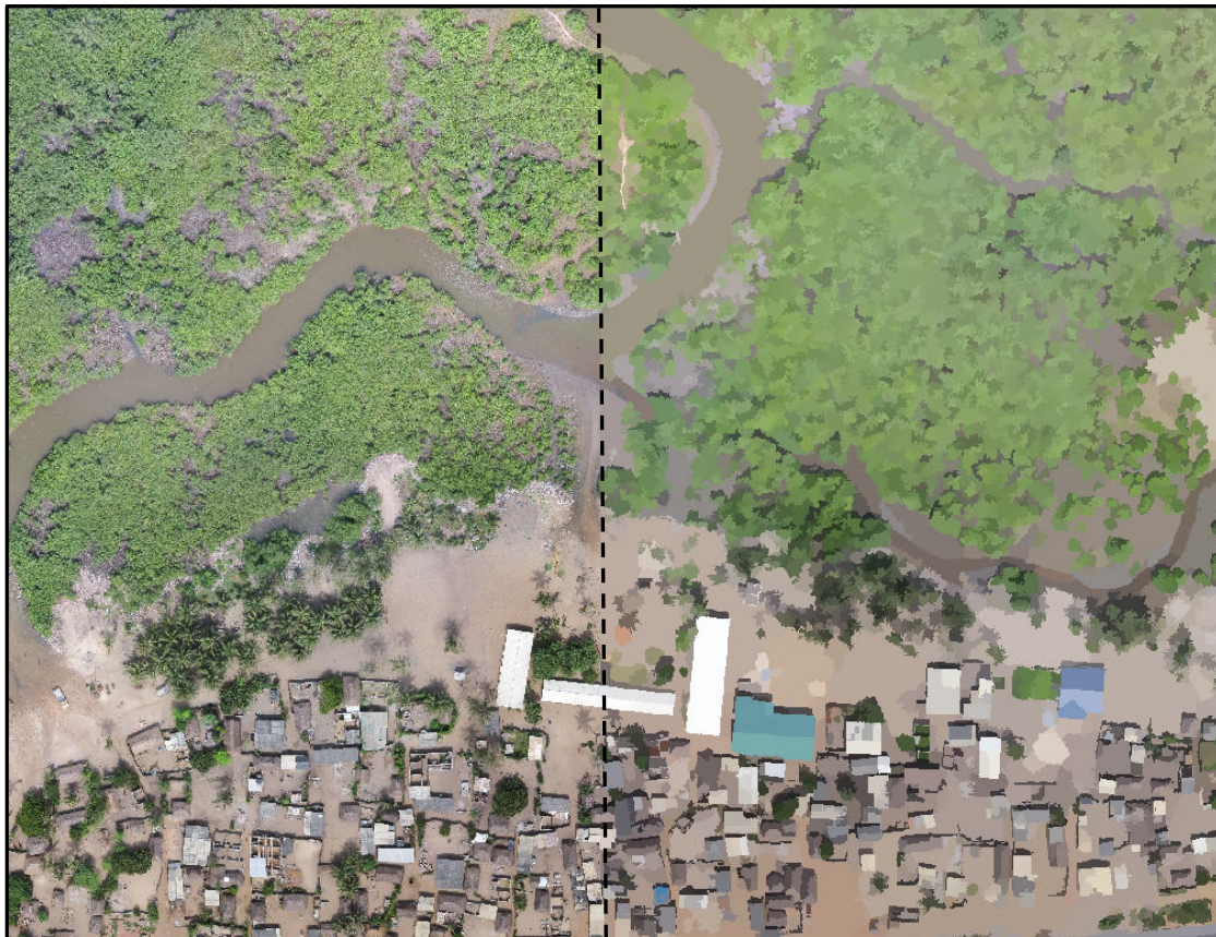
Figure 15 A subset of the Iture image mosaic displaying the original image (left) alongside the results from the image segmentation process (right).
