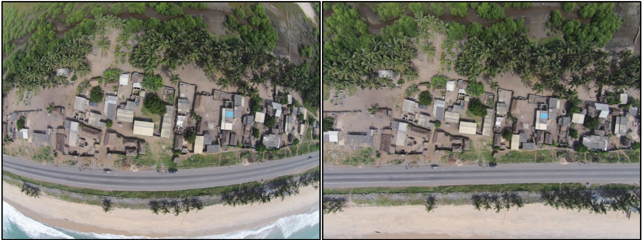
Figure 5 An example of a raw UAV image (left) showing the effects of fisheye distortion caused by the wide angle lens, and the same image after the distortion has been removed (right) during post processing.
