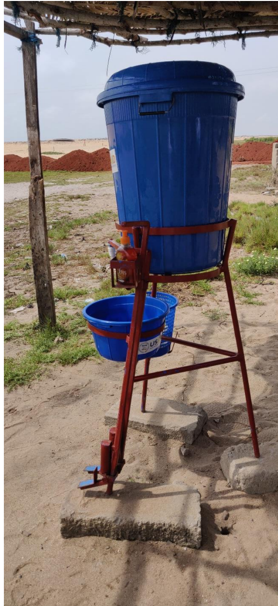
Figure 4 Handwashing station and stand at Whuti repainted with Anti-rust paint
