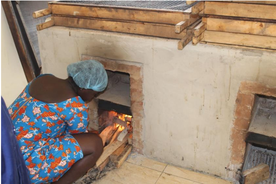
Figure 6. Facilitator explaining the importance of Grate in the Ahotor Oven
