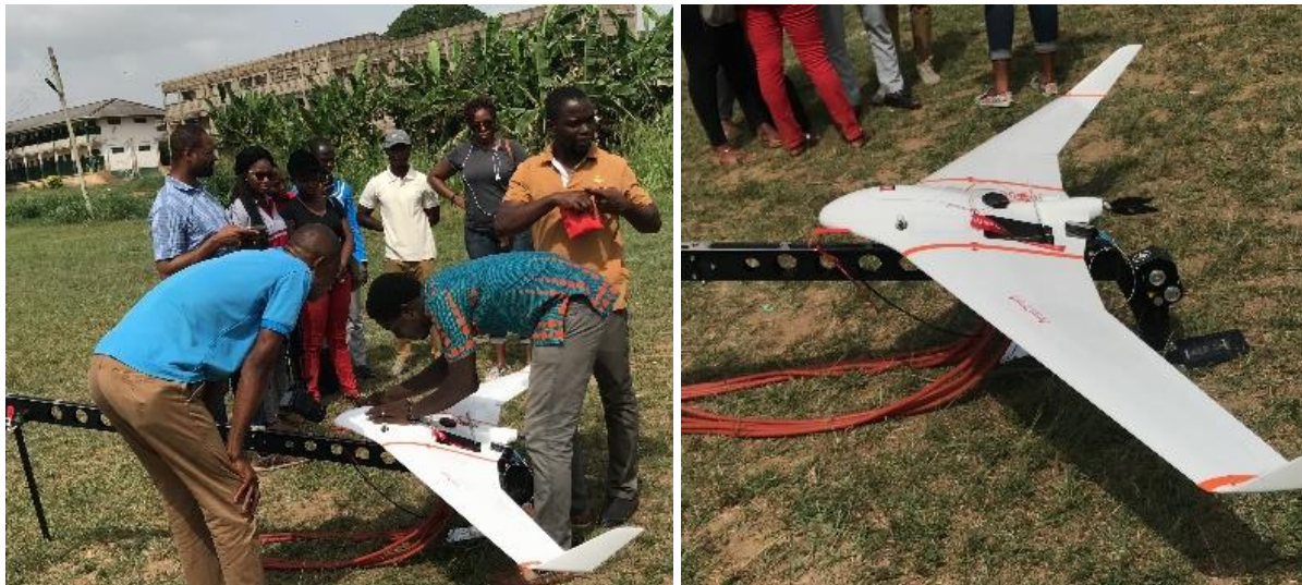
Figure 12: Use of the Bramor to map coastal water bodies along the coast of Ghana
