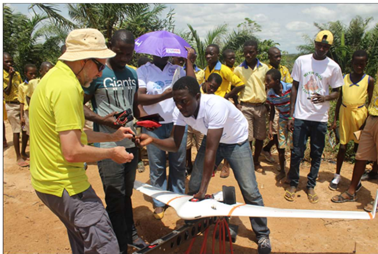
Figure 12. Prepping the unmanned aerial vehicle for a flight to collect land cover imagery in the Pra River estuary and surrounding wetlands. (Photo credit: Gloria Otoo, CSLP)
