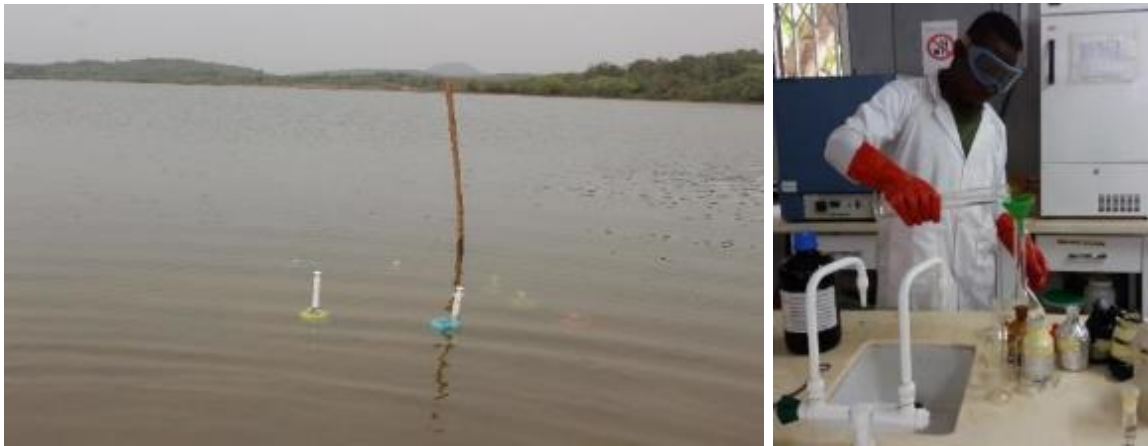
Figure 44: Field experimental setup for nutrient flux determination at Sumina Lagoon (left). Student preparing reagent for laboratory analysis of samples (right)
