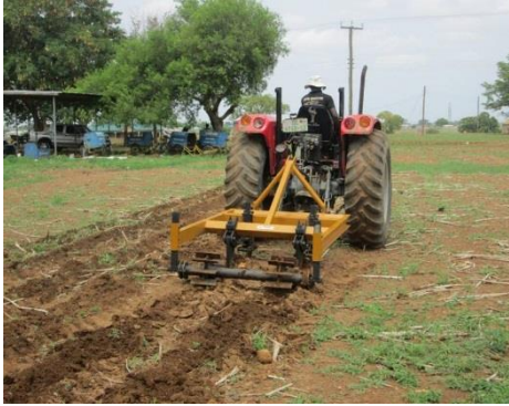
A demonstration on the use of a ripper - one of the climate smart interventions that prevents soil depletion
