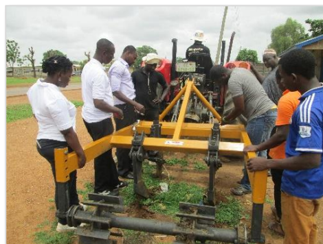
Picture 5: Setting the ripper with operators and farmer at Aramkoliga, UER
