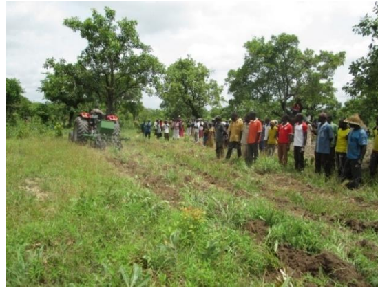
Outgrowers observing the operation of the ripper during land preparation
