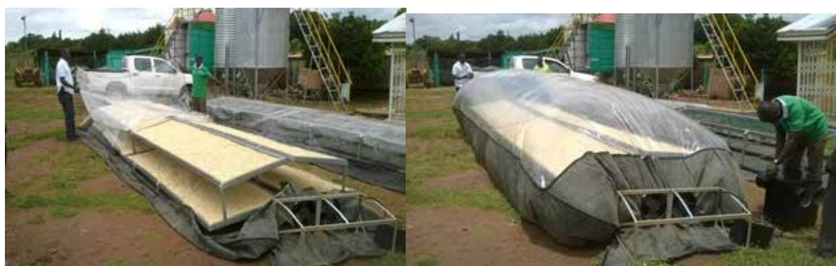
Picture 4. 4: Fully covered Work View (left) and locally Manufactured Solar Hybrid Balloon Dryer (right)
