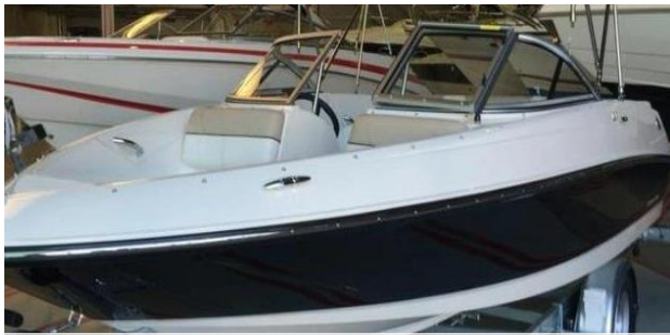
USAID/UCC Project Research Boat Bayliner 175BRE fibreglass boat with 135hp Mercruier WPS Engine - 5.36 metre long
